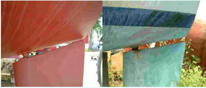
Two rudders, two Westerly Centaurs, the one on the left has a bent ruder stock
