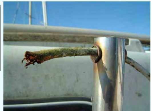
Corroded lifeline..not a lifeline you would trust your life to!
