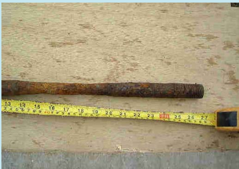
A 1" diameter keelbolt with a degree of "Waisting"
