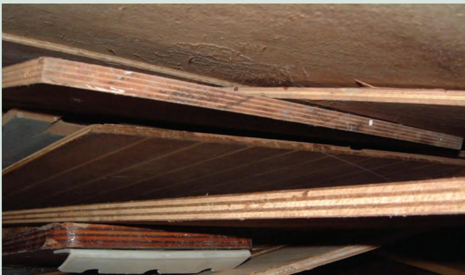
Various sheets of plywood, note the differing veneer construction, the more veneers the stronger, particularly if all veneers are the same thickness
