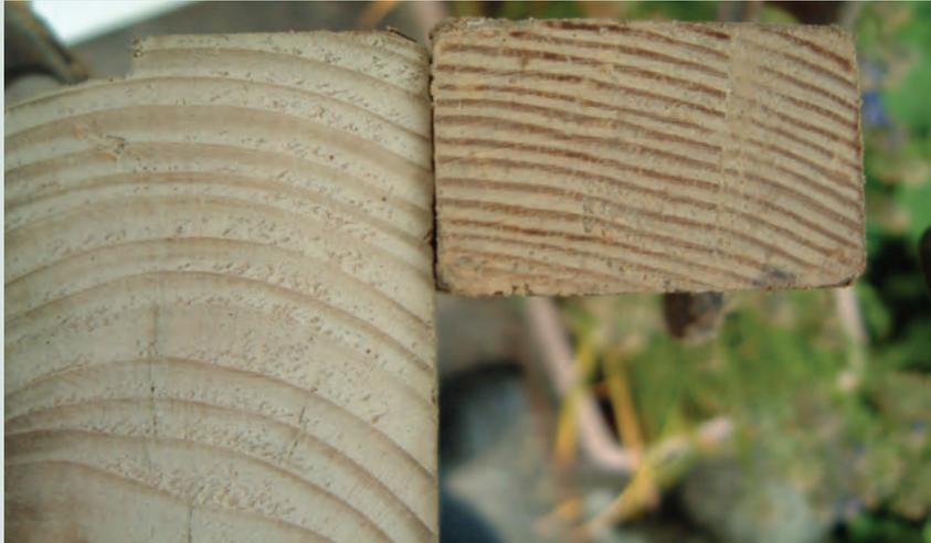
Two sections of pine, on the left fast grown, fewer rings much lighter in weight, on the right slower grown heavier & stronger, almost twice as many rings for the same section size
