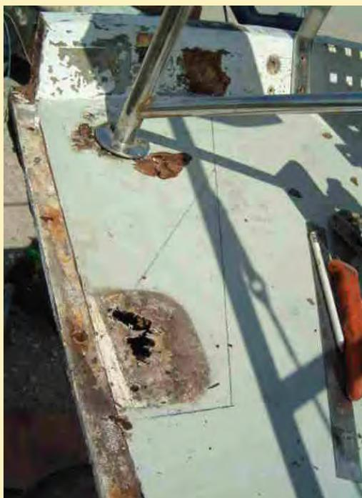
The main drawback of plywood is that it is nowhere near as resistant to fresh water decay and deterioration as solid timber once any breach has been made where water can leak into the edge of plywood and, with a plywood deck, it is obvious there are extremely long vulnerable edges that have to be sealed.
