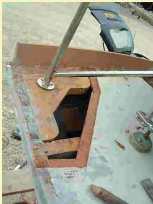
Here can be seen a series of discovering the rot, replacing all the underlying quarter knee that had completely disintegrated and the final finishing. This was caused by water leaking in the pushpit fastenings
