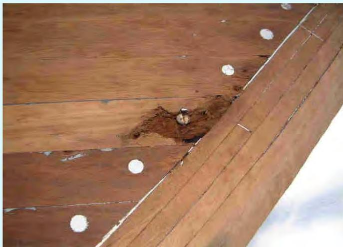
Note the narrow strips and laminated stem. Note the decay in one hood end
