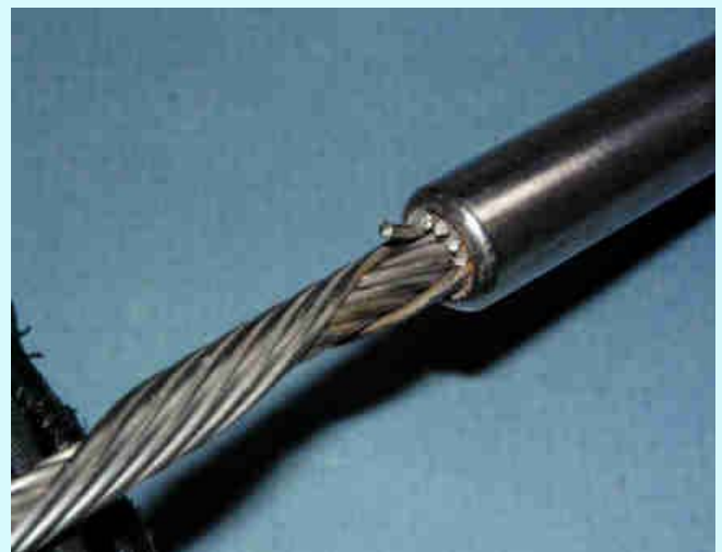
Stainless wire showing work hardened & broken strands at the swage. Galvanised does not suffer the same fault generally
