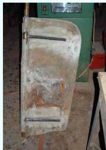
Internals of bronze stock/ mild steel tang rudder
